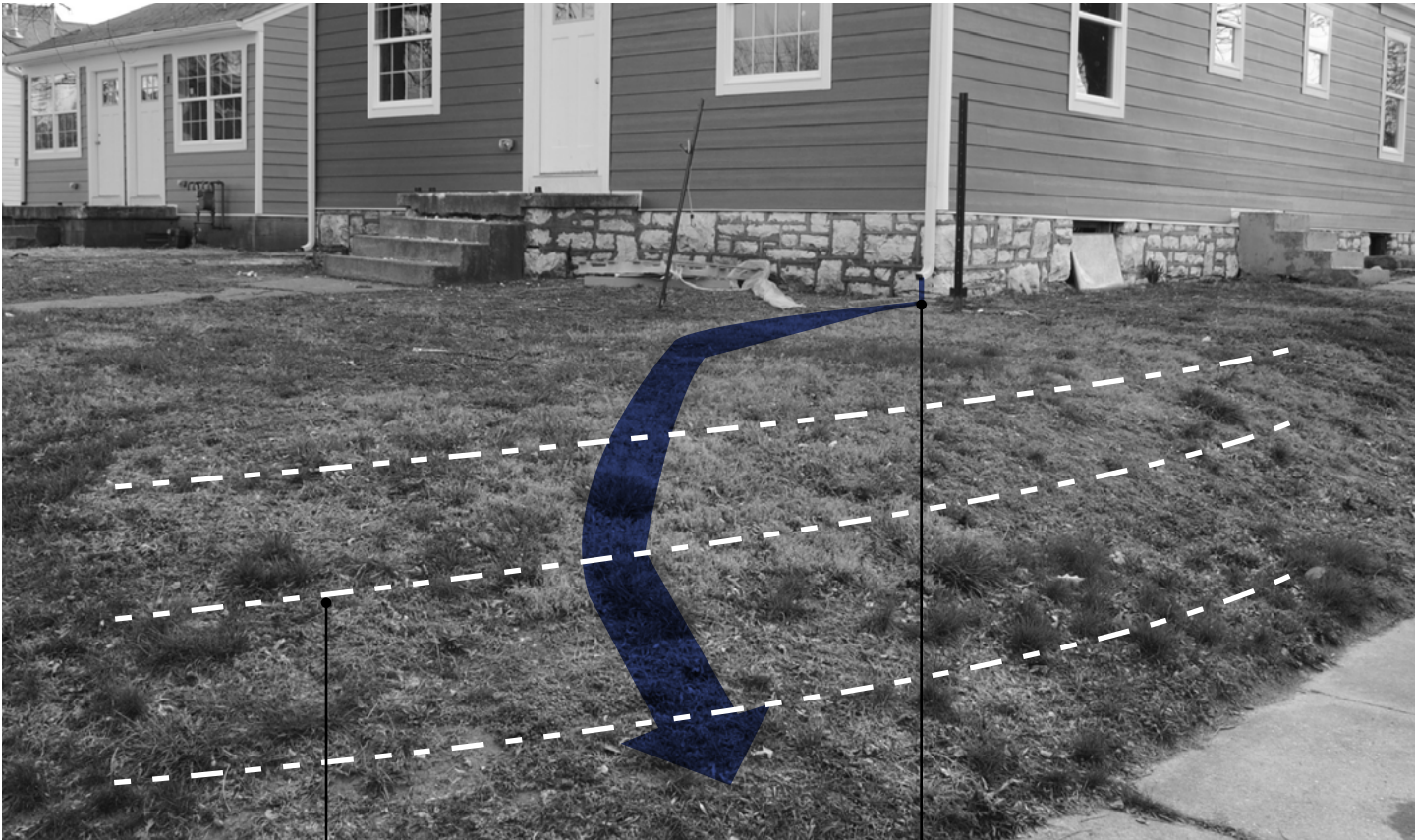
Stormwater runs directly off the steep lawns into the adjacent sidewalks, eroding the yard and flooding the right-of-way.
