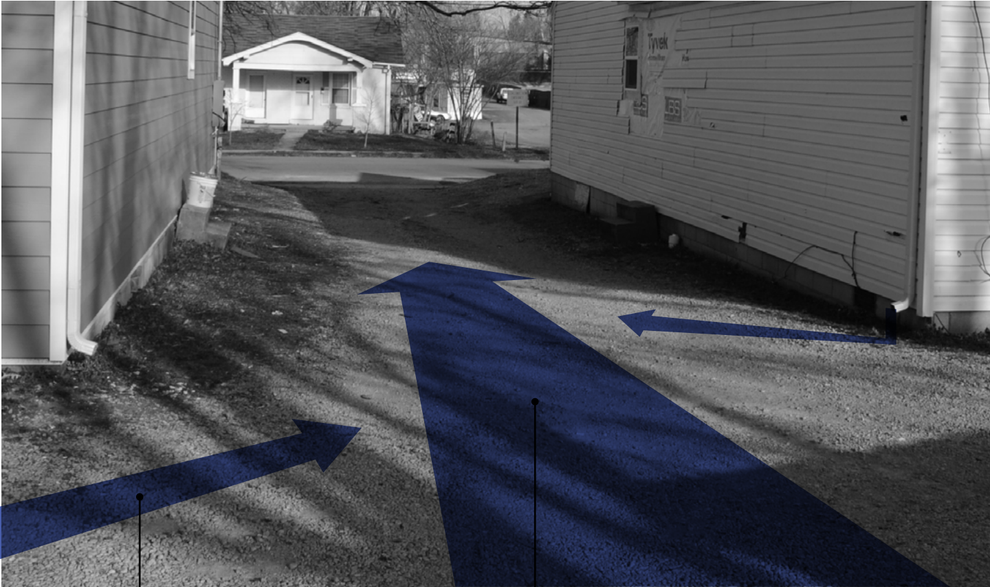
Stormwater runoff from downspouts adds to overflow along the central drive, playing a key role in flooding issues along the main frontage road.
