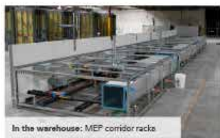
In the warehouse: MEP corridor racks
