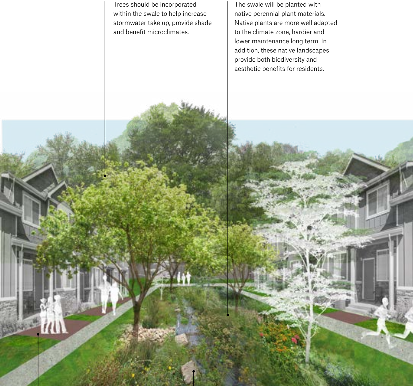
The swale will feature river stone as an aesthetic element that also slows water down and helps provide a limited amount of short-term storage capacity in void spaces.
